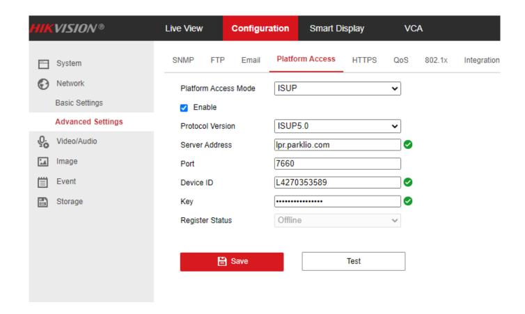
After entering the information click the Save button to apply changes. To test if the settings were entered correctly click on the Test button. If no error was found a Test successful message will be displayed and the camera Register status should change to Online. After setting up the camera, navigate to the ANPR page on the Parklio PMS, and the camera should be connected and online.
