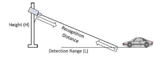
Select a proper lens according to the table below. The identification distance is based on the camera's focal length.
