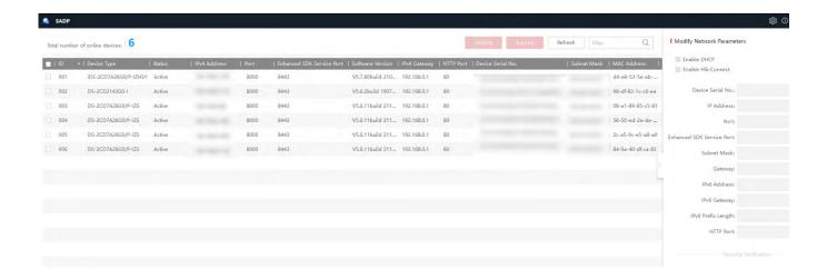
Once the SADP tool is open any cameras that have not been setup will appear as Inactive.
