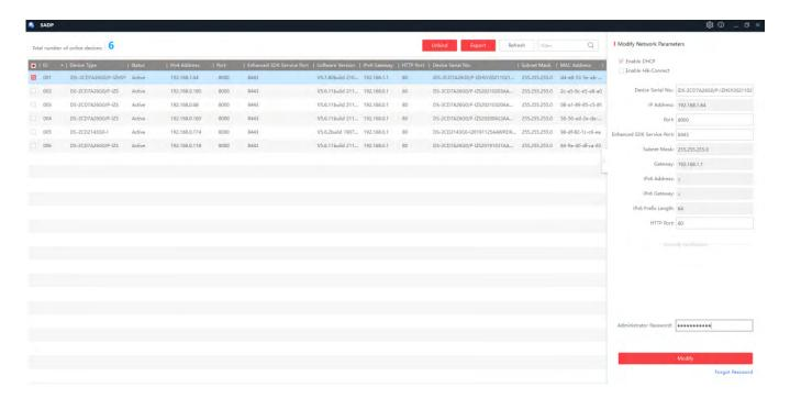
NOTE: If a static IP address is required, the SADP tool can be used to configure a static IP address and network parameters by disabling DHCP and entering network parameters.
